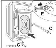
**6.** Open the porthole, take out the inlet hose from the drum and remove the polystyrene block fitted on the door seal.
